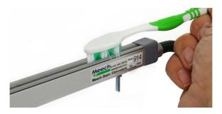
lonising bars will need periodic wiping to clean grey deposits from the surface of the bar. A cloth moistened with a small amount of IPA or methylated spirits is recommended.
