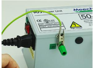
■ Holding the wire insulation, approach any of the bar emitter pins with the bare end of the wire or metal clip end.
