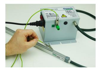
As the pin is approached, a small faint spark should jump from the pin to the wire.
