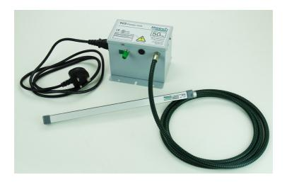
The Power Unit converts the electrical supply into a high voltage, low amperage output. This output energy is transferred to the 914 bar by the HT cable.
