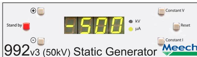
Display with 992v3-50kV operating in Constant Current Mode
