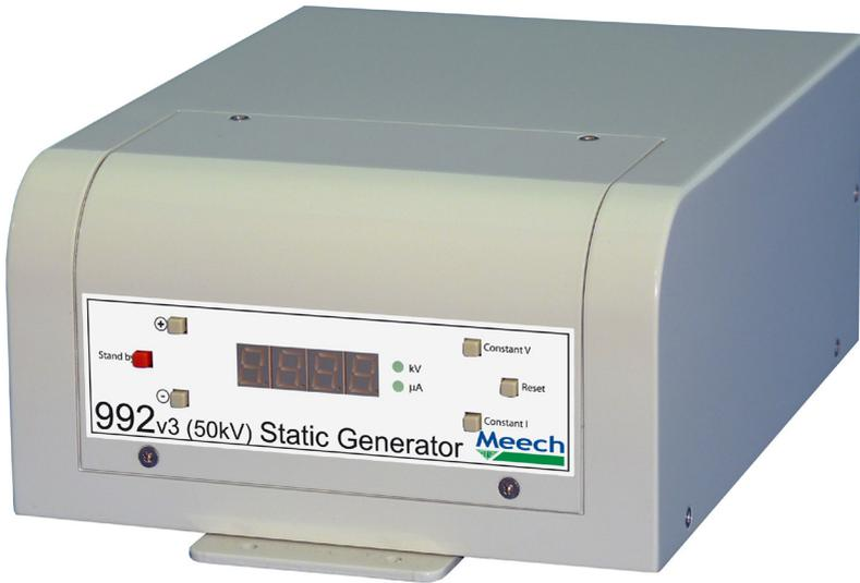
The Model 992v3-50kV Static Generator can be set in either Constant Voltage or Constant Current Mode to create a controlled level of static charge to impart temporary bonding (static pinning) between materials, at least one of which is insulative.
