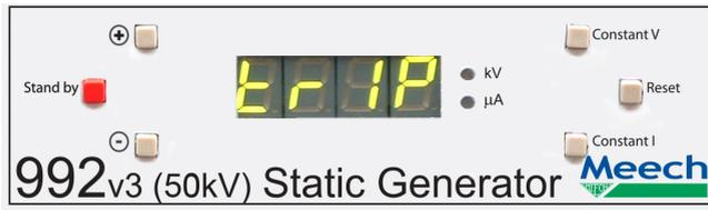
Display with 992v3-50kV “Tripped” out
