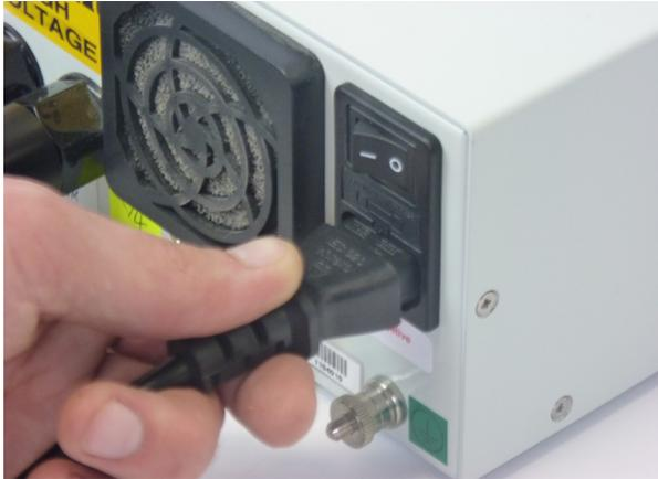
The generator is fitted with an internal switchmode power supply; thus any voltage from 85 to 265V, 50Hz or 60Hz, can be supplied to the unit.
