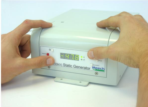
To adjust the output voltage (adjustable from 0 - 50kV), press and hold the Constant V, and use + and - to adjust the set voltage.
