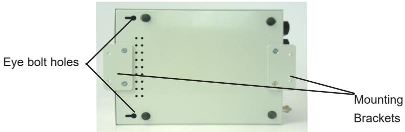
It is also possible to mount the 992v3 (50kV) vertically using the eye bolt holes and mounting bracket provided. (See mounting details at the end of this manual for eye bolt positions). When mounted vertically the front control panel should be removed by unscrewing the 4 retaining screws and refitted as shown in the photos overleaf.
