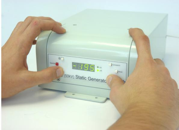
To adjust the current limit (adjustable from 0 - 260 $\mu$ A), press and hold Constant I and use + and - to adjust the current limit. When the Constant I button is released the display will show the actual current being drawn by the system.
