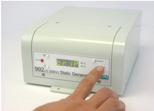
When the 992v3-50kV has tripped, it can also be reset by switching off power to the 992v3-50kV at the mains IEC switch and switching it back on again.
