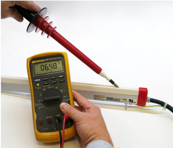
6. If the voltage is below 4.0 kV then the bar should be returned to Meech for service and/or repair.
