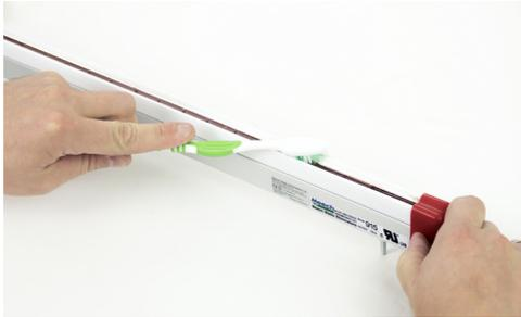
Ionising bars will need periodic wiping to clean grey deposits from the surface of the bar. A cloth moistened with a small amount of IPA or methylated spirits is recommended. Allow a moment to dry before switching on.
