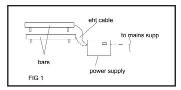
The Power Unit converts the primary electricity supply into a high voltage, low amperage output. This output energy is transferred to the Meech bar by the HT cable. A capacitive coupling inside the bar reduces the energy at the ionising pin to a level which is completely shockproof to a human being.
