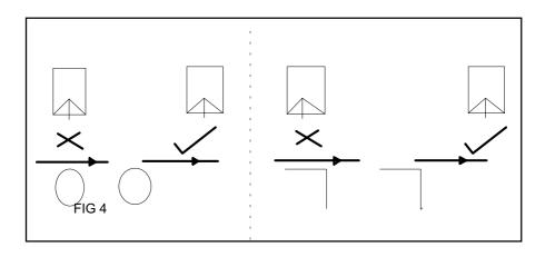
3. Avoid proximity to earthed parts of machine as this will distort the corona and reduce its efficiency.
