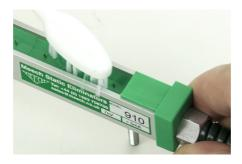
lonising bars will need periodic wiping to clean grey deposits from the surface of the bar. A cloth moistened with a small amount of IPA or methylated spirits is recommended.
