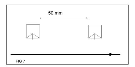
4. If bars are needed on each side of the material, they should be staggered.
