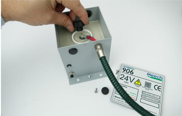
Before Re-attaching the lid using the two screws removed in stage 1 make sure all of the nuts are fully tightened before the lid is attached.
