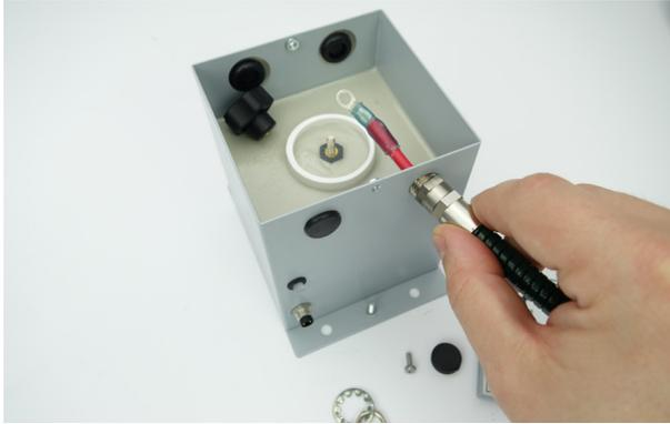
Push the connector through a port in the Hyperion power supply. Re fit the lock washer and nut to secure the appliance cable. Make sure the nut is fully tightened.
