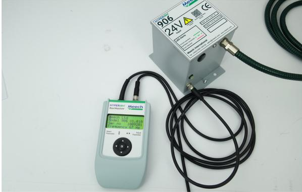
The BarMaster is connected in line with the 906's power supply cable. The power cable is connected to the BarMaster and, in turn, its cable is connected to the Hyperion 906 Unit.
