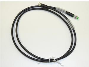
Power Cables and Power Extension Cables - 4 Pin M8 (straight or 90° elbow) available in 1, 3 or 8m lengths.
