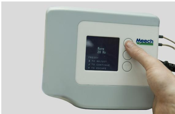
If the bar is positioned a long distance from the target area (600mm-750mm) the “Rate” should be set to the lowest setting. If the bar is positioned close to the target area (150mm -300mm) the “Rate” should be set towards its maximum.
