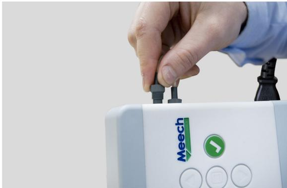
Connect the mains supply to the Pulsed DC Controller and switch ON. The 971 Bar will now produce Pulsed DC ionisation from the emitters of the bar.
