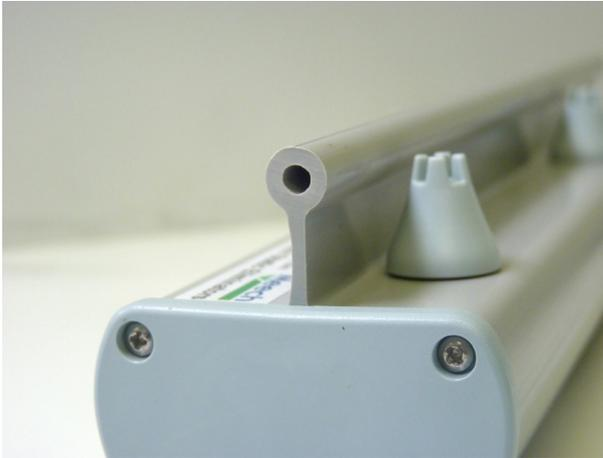
The upstand between the nozzles is a vital feature of the 971 bar. By increasing the tracking distance between positive and negative pins, the upstand helps maintain good performance even when the bar is contaminated.
