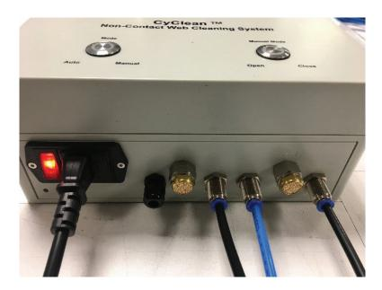
The compressed air hoses (blue and black) should be connected from the CyClean unit to the 6mm compressed air push fittings labelled Port 2 and Port 3. The blue hose connects to port 2, the black hose connects to Port 3.
