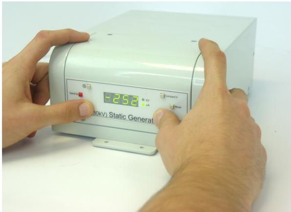
To adjust the current limit (adjustable from 0 - 500 $\mu$ A), press and hold Constant I and use + and - to adjust the current limit. When the Constant I button is released, the display will show the actual current being drawn by the system.
