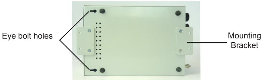
It is also possible to mount the 992v3 vertically using the eye bolt holes and mounting bracket provided. (See mounting details at the end of this manual for eye bolt positions). When mounted vertically the front control panel should be removed by unscrewing the 4 retaining screws and refitted as shown in the photos overleaf.
