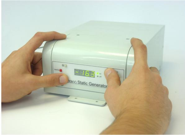
To adjust the output voltage (adjustable from 0 - 30kV), press and hold the Constant V, and use + and - to adjust the set voltage.
