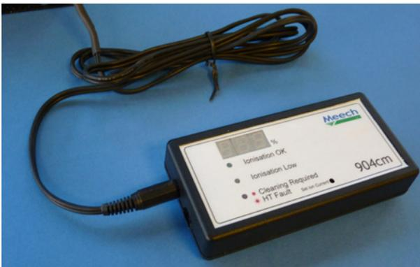
Ideally the unit will be positioned where it can be seen easily by the operator. The magnetic strips on the rear of the unit allow it to be mounted easily on any steel surface.
