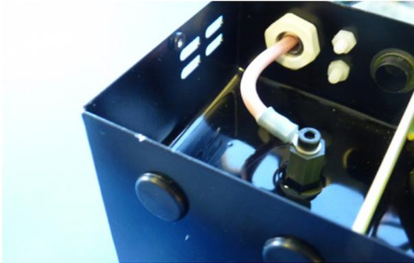
The 904CM monitoring unit is connected to the 904 Power unit using the signal cable provided. At the power unit, connection is made using the socket in the power unit wall with the trailing wire connected to the earth terminal.
