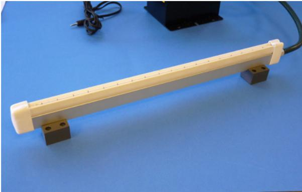
For correct operation the 915 ionising bar(s) must be mounted using the insulating mounting blocks supplied by Meech. The bars must not be grounded at any point.
