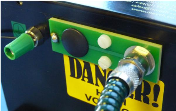
For correct operation of the monitoring system, the conduit from the ionising bar(s) must be connected using the modified connection plate.
