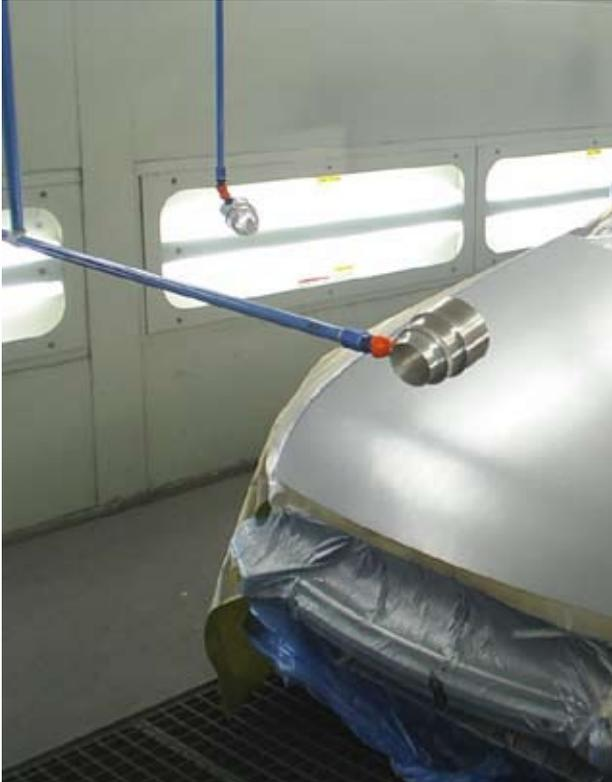
The 14 drop points give complete freedom to set up the Air Amplifiers in a variety of configurations to suit the particular item or items to be dried. For example the system can be set up to dry a panel still fitted to the vehicle at the same time as drying other panels on stands.
