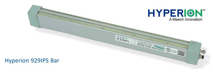
The Hyperion 929IPS is a compact mid-range pulsed DC ionising bar. Powered by an internal 24V DC power supply the 929IPS is designed to be easily installed onto printing and converting machinery. The class-leading +/-10kV pulsed DC output provides extremely powerful ionisation. The bar features Meech's Ion Current Monitoring (ICM) technology, this ensures performance is maintained with local and remote alerts cleaning is required.
