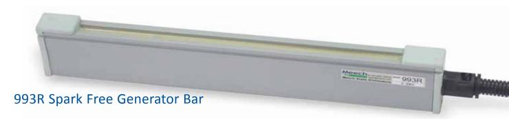
The 993R is a high performance generator bar used with the Meech range 992V3 30kV and 50kV Static Generators. Resistively coupled emitter pins deliver smooth, controlled pinning whilst spark free operation avoids tripping out on intermittent applications.
