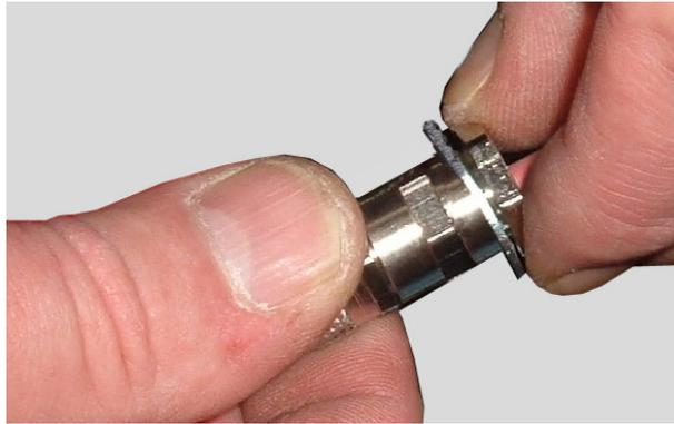
Push the connector through a port in the power supply adjacent to the high voltage terminal.
