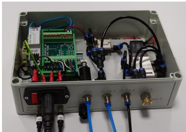
The compressed air hoses (blue and black) should be connected from the TakClean unit to the 4mm compressed air push fittings labelled Air Out 1 and Air Out 2. The blue hose connects to Air Out 1, the black hose connects to Air Out 2.
