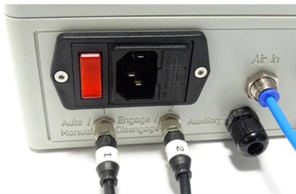
Connect plug 1 from the TakClean to the Auto/Manual socket on the pneumatic control box.
