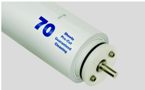
6. Fit the core chuck assemblies to a new roll of adhesive material. Be sure to fit the core chuck assembly flush into the new adhesive roll and to tighten the 2 bolts on each core chuck assembly. The core chuck assembly grips the inside of the core by expansion ring friction, therefore the bolts should be tight.
