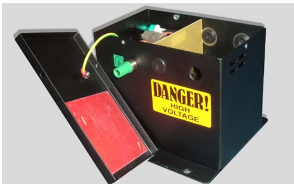
Connect the ionising bars by removing the lock washer and nut from the swivel connector of the appliance.
