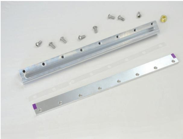
Do not over tighten the M6 bolts and crush the shims. All bolts should be tightened to a maximum of 4Nm or 2.95f/lbs.
