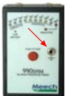
Place the meter on the surface being tested. Connect the meter to a known ground through the ground connection located near the test button. NOTE: When the ground wire is connected through the ground jack, the meter will not measure surface resistivity. Press the centre button labelled "TEST" and the LED will illuminate to indicate the resistance to ground. If the LED labelled "INSULATIVE" illuminates, the resistance to ground of the surface under test is greater than  $10^{12}$  Ohms.
