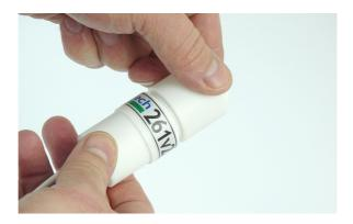
Typically, weekly cleaning is sufficient. However, equipment used in some heavy contamination areas, such as gravure printing or where plastic fumes are present, may require daily cleaning.
