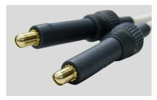
If you find this to be the case, then (1) if the plugs are too tight, you should lightly pinch together the two halves of the brass end of the plug with a pair of pliers, or (2) if the plugs are too loose, you should gently open out the slot in the brass end with the blade of a screw-driver or knife.
