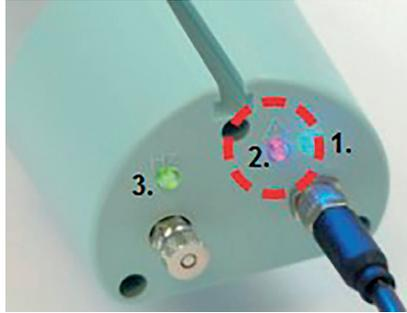
When the equipment powers on, the (1.) Blue LED will illuminate and the (3.) Hz LED will start to flash red and green in time with the Hz setting. If (2.) Warning LED starts to flash or is solid red, check the ion level with the BarMaster.
