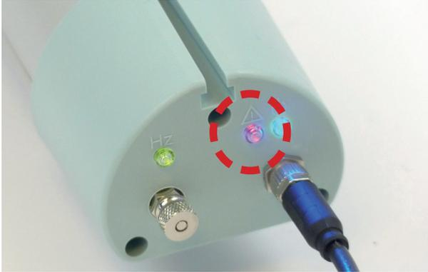
Red flashing LED shows that bar is dirty and needs cleaning. Solid red illumination indicates a fault with the high voltage output.
