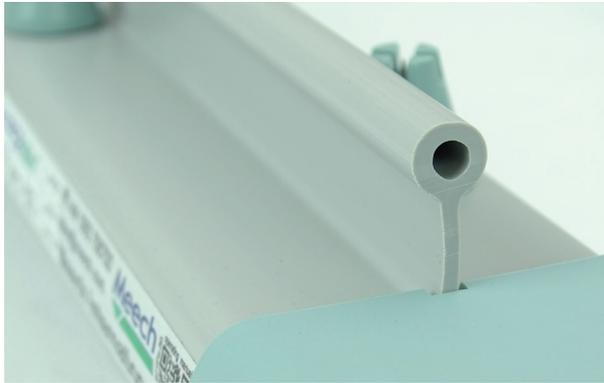
The divider used on all Meech pulsed DC bars is an essential feature that ensures good operation in dirty, factory environments. To maximise the interval between cleaning the 9711PS-30 bar features a divider to increase the surface tracking distance between the two rows of high voltage pins. It is important to clean this area during cleaning operations.
