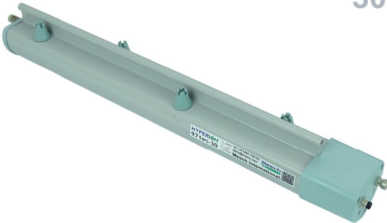
The Hyperion 971IPS-30 is a powerful, very high voltage pulsed DC ionising bar. It is used to control static electric charges in long to extra long-range applications (450-1500mm). An integral 30kV pulsed DC power supply allows for easy installation on extrusion, converting and packaging machinery. Requiring only a 24V DC supply, the 971IPS-30 removes the need to route high-voltage cabling through the machine.
