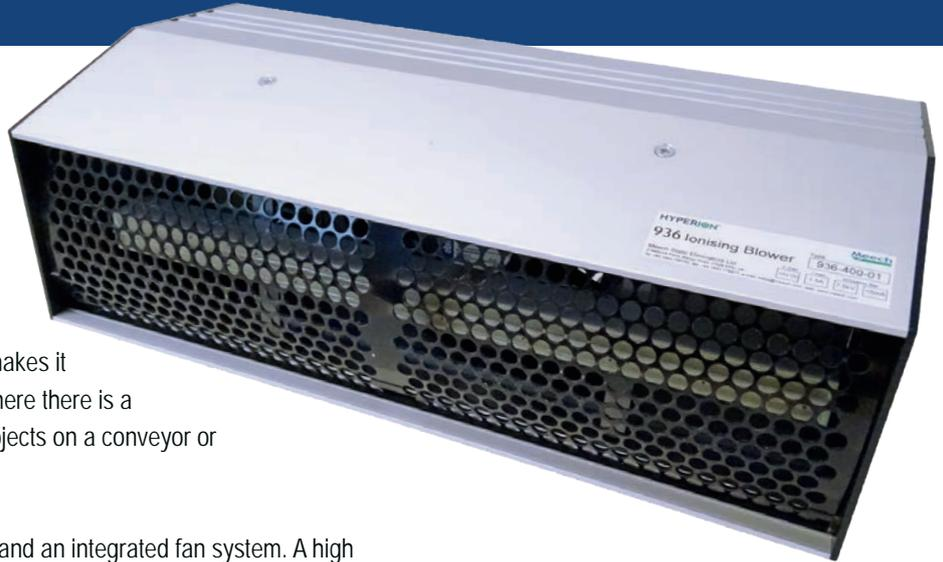
The 936 Blower is comprised of an ionising head and an integrated fan system. A high volume flow of ionised air is generated by blowing air through the ionisation head at the mouth of the unit. Ionisation is provided by the 924IPS bar, generating an operating range of up to 1200mm.
