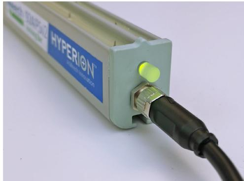
The 924IPsv2 is powered by 24V DC via a 4-pin M8 Connector.
