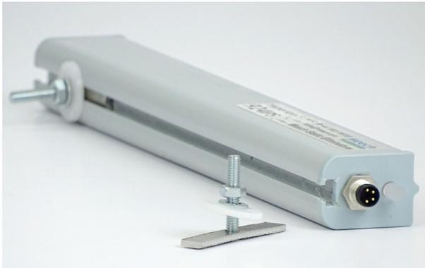
The bar is mounted using the T-Slot at the rear of the bar. M4 T-bolts supplied with the bar may be positioned to suit convenient mounting points.
