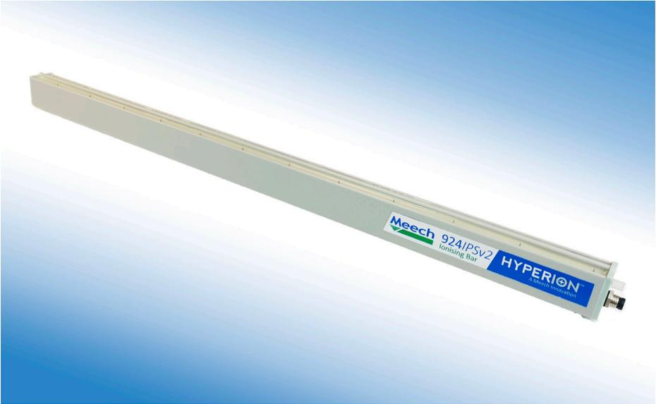
The Hyperion 924IPsv2 is a compact pulsed DC ionising bar. It is used to control static electric charges in short range applications (20-150mm). An integral 7.5kV pulsed DC power supply allows for easy installation on printing, converting and packaging machinery. Requiring only a 24V DC supply, the 924IPsv2 removes the need to route high-voltage cabling through the machine.
