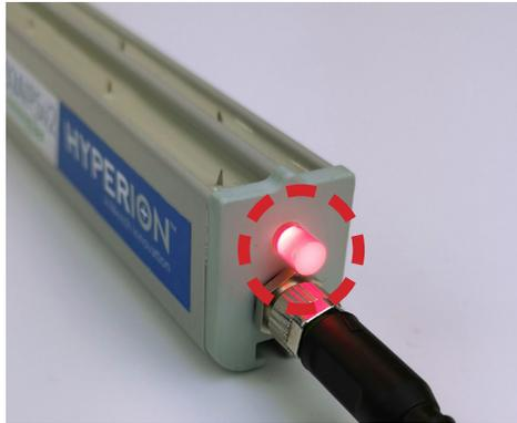
The local LED illuminates constant green to indicate that the bar is on and working correctly. Red flashing LED shows that bar is dirty and needs cleaning. Solid red illumination indicates a fault with the high voltage output.
