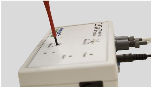
When set to SSDC mode the effective range of ionisation is up to 200 mm from the ionising bar.
