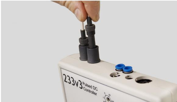
3. Connect the 24VDC input supply to the controller and switch ON. A Mains lead for the Meech switch mode power supply is provided. The mains supply to the switch mode must be electrically grounded.
