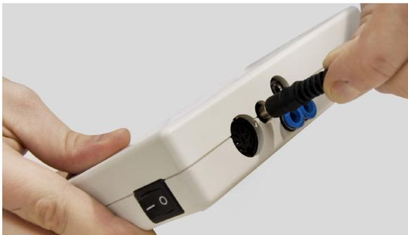
If using anything other than the Meech 24V supply please note the zero volt (0V) must be electrically grounded (connected to earth).
