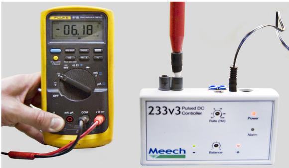
5. If the controller is found to be functional, test each of the attached products independently following the instructions detailed in the appropriate Operation and Maintenance manual.
