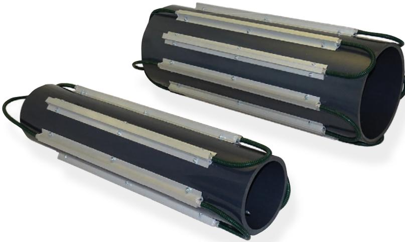
The 913 Flow Tube neutralises static charges on materials in handling and conveying systems. It incorporates in-line ionisation, which eliminates material clinging and clogging in ducting systems due to static charges. The 913 Flow Tube is powered by 905 power supply and is provided in a range of diameters to fit most of the industrial standard installations.
