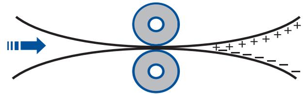
Charging by separation also occurs when two materials' surface electrons are in close proximity. Upon separation of the materials, electrons have a tendency to adhere to one material or the other, dependant on the material composition. Similarly, the level of charge can be affected by the speed of separation: the faster the separation, the higher the charge and the slower the separation, the lower the charge.
