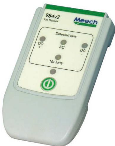
The 984v2 Ion Sensor is a device used for checking the performance of both AC and DC powered static elimination bars. Indicator lights confirm the presence of ions, and in the case of a DC power source their polarity. Regular monitoring of installations with the 984v2 will indicate when bars require cleaning or other maintenance work.
