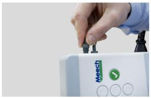
11. Reconnect the supply and switch on the unit.
